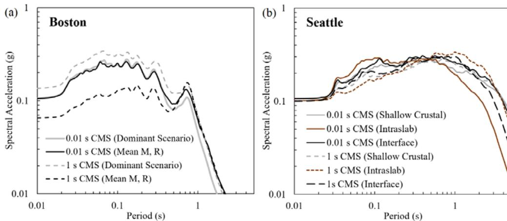
Figure 6. Predicted surface response spectra from nonlinear site response analyses for the medians of various suites of ground motions in (a) Boston and (b) Seattle.
