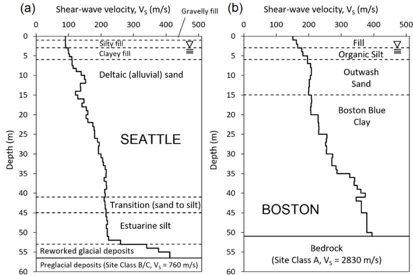
Figure 1. Shear-wave velocity profiles and stratigraphic profiles used in the analyses for (a) Seattle and (b) Boston. The groundwater table was assumed to occur at a depth of 3 m at each site.
