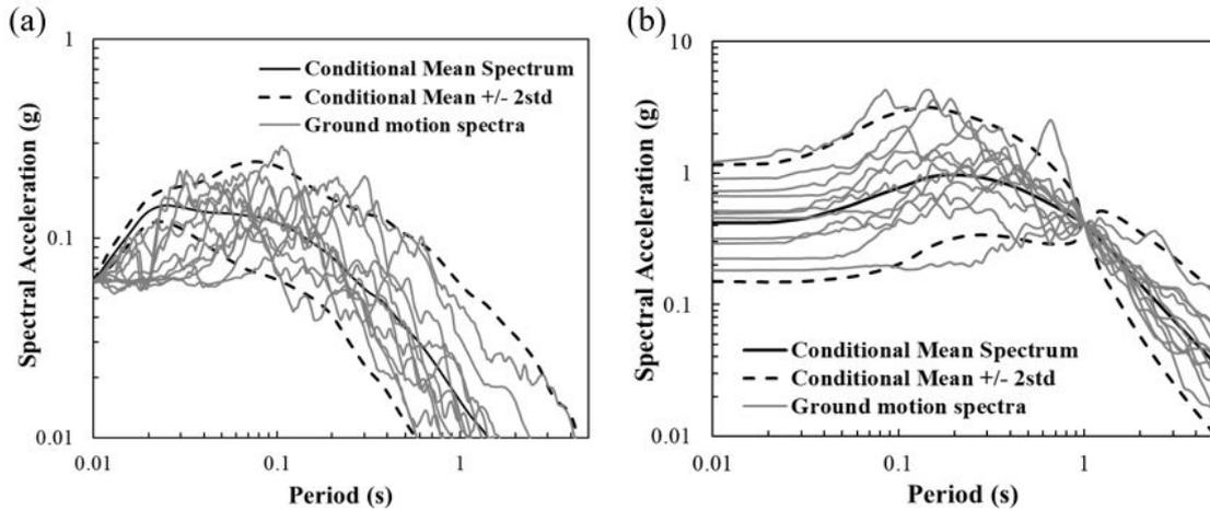
Figure 5. 5% damped response spectra of selected ground motions matching the CS for (a) Boston for  $T^*=0.01$  s (selected dominant scenario) and (b) Seattle for  $T^*=1.0$  s (shallow crustal dominant scenario).
