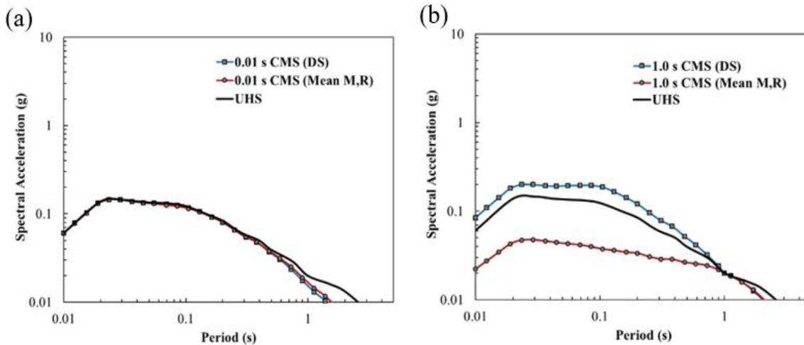
Figure 4. UHS and CMS at Boston for selected scenarios (M-R combinations) for conditioning periods of (a) 0.01s and (b) 1s.
