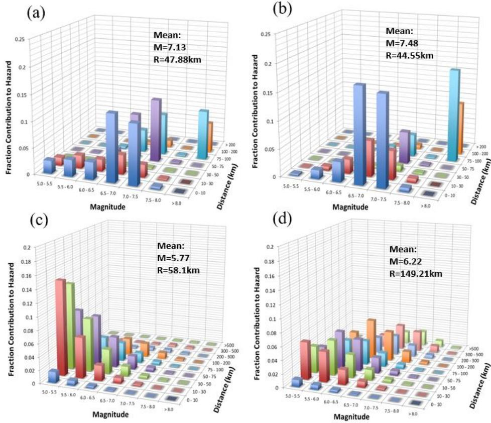
Figure 2. Seismic hazard deaggregation plots for spectral accelerations exceeded with 2% probability in 50 years at (a) Seattle for 0.01s period, (b) Seattle for 1s period, (c) Boston for 0.01s period and (d) Boston for 1s period.
