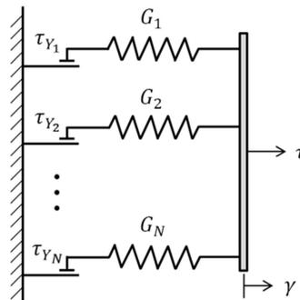
**FIG. 1. Schematic of the Iwan (1967) and Mroz (1967) material model composed of elastoplastic springs in parallel.**
