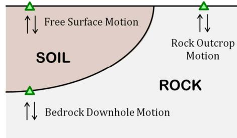
**FIG. 4. Illustration of site response terminology, showing the free surface motion (above a soil profile), rock outcrop motion, and bedrock downhole motion.**
