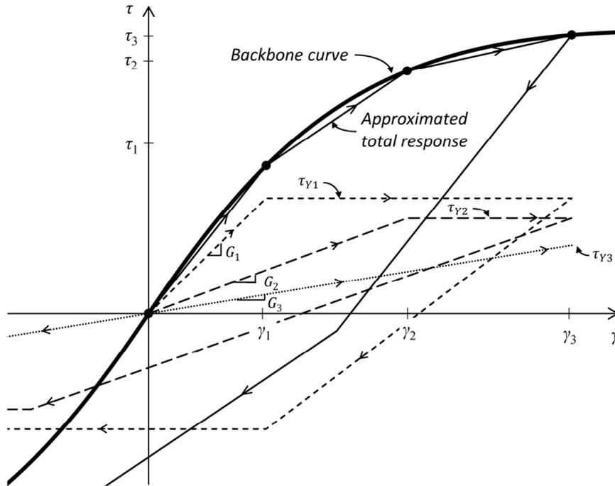
**FIG. 2. Stress-strain behavior for  $N = 3$  elastoplastic elements in parallel. Dashed lines indicate the stress-strain behavior of each element, and solid lines indicate the total stress-strain response of the material.**
