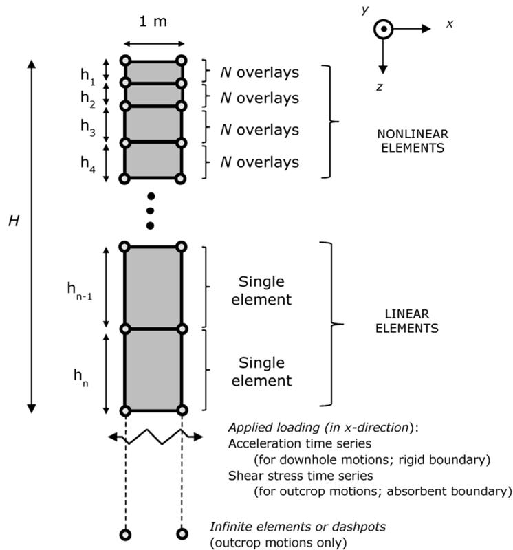
FIG. 3. Schematic of the finite element model for earthquake site response.
