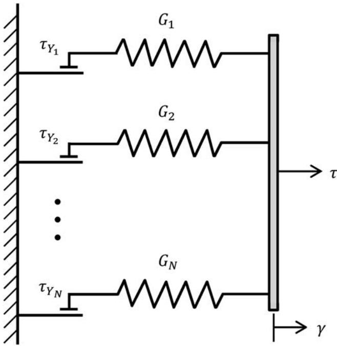
▲ **Figure 1.** Schematic representation of the 1D Iwan (1967) and Mroz (1967) material model (IM67) composed of elastoplastic springs in parallel.
