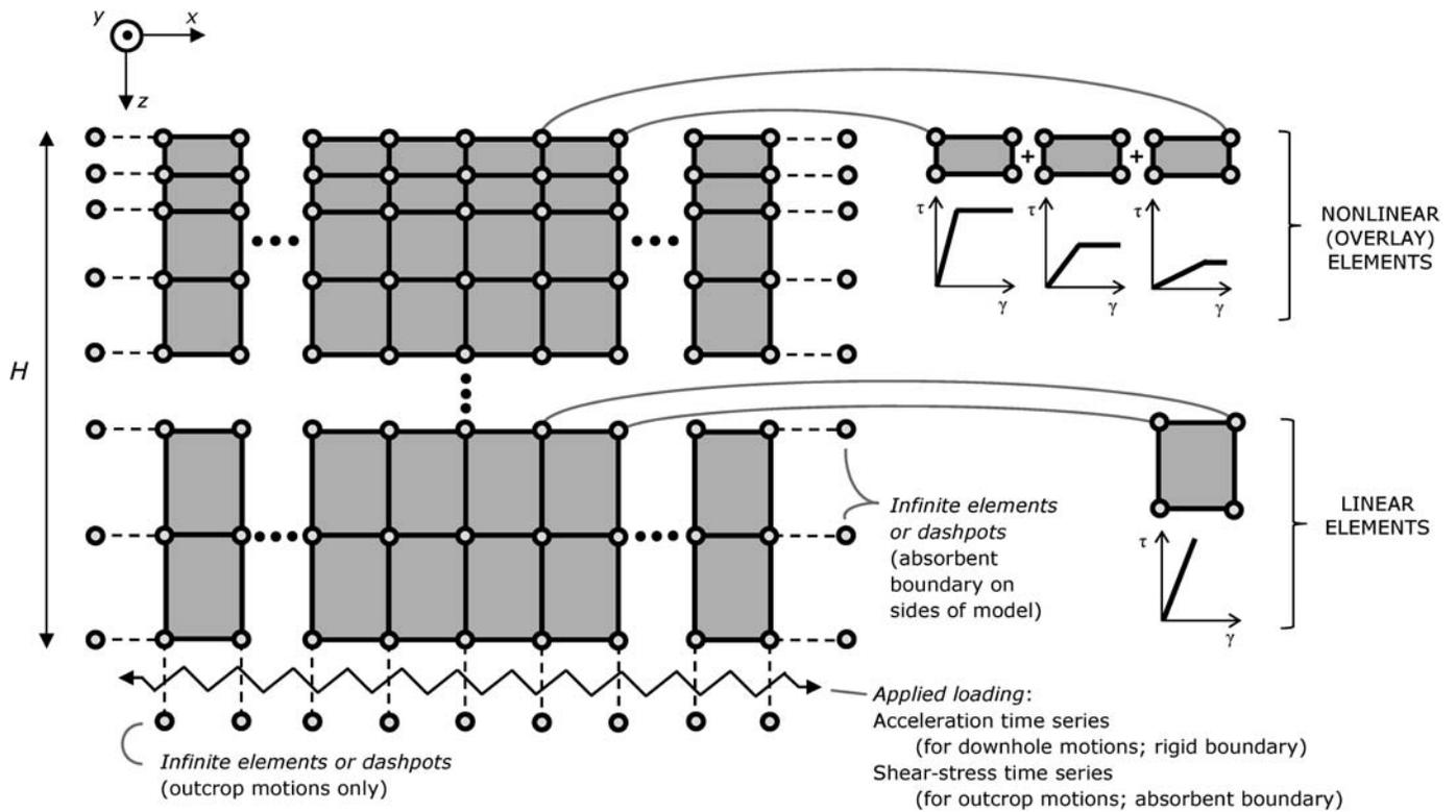
▲ **Figure 6.** Generalization of the overlay model to represent 3D site-response behavior. The model is symmetric in the  $x$  and  $y$  directions (the  $y$  direction is out of the plane of the page and not shown). On the sides of the model, infinite elements or dashpots are required to establish an absorbent boundary scheme. At the bottom of the model, like the 1D case, infinite elements or dashpots are used when the input motion is obtained from an outcrop recording.
