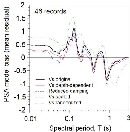
**Figure 6.** NL model bias (mean residual) as a function of spectral period for the alternative physical hypotheses, using the 46 ground motions at FKSH11.
