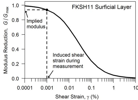
**Figure 3.** Illustration of the potential measurement bias in  $G_{max}$ , using the assumed modulus reduction curve of the surficial layer at FKSH11. If the surface-downhole test induces  $0.001\%$  strain in the soil, then the associated shear modulus is actually less than the true  $G_{max}$ .
