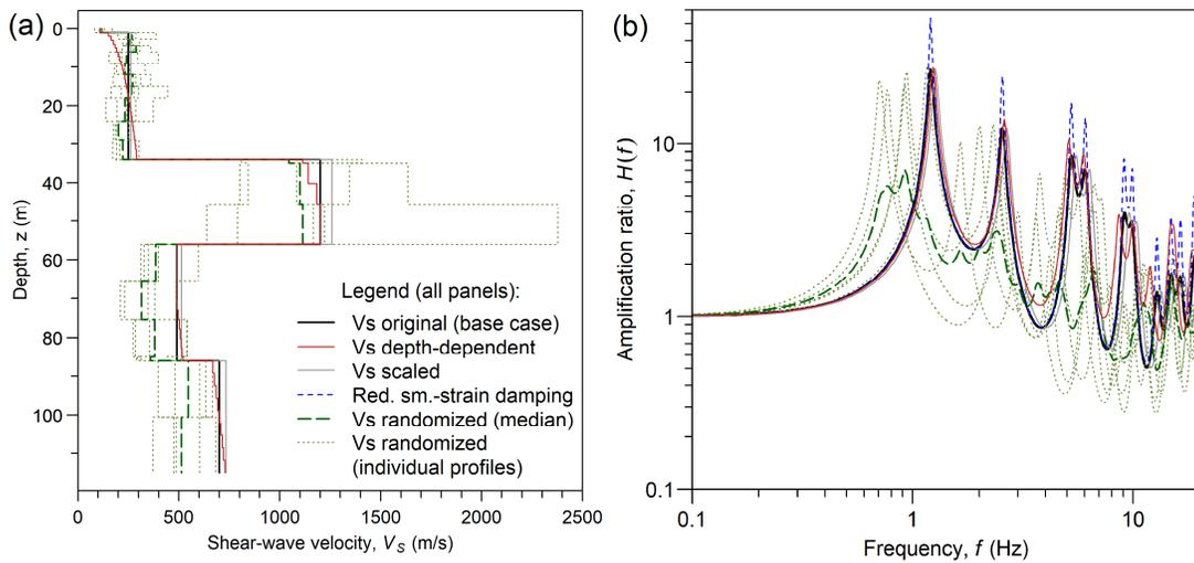
**Figure 4.** Results of the adjustments to the soil profiles and constitutive model parameters at FKSH11; (a)  $V_S$  profiles, and (b) theoretical 1D linear amplification spectra for the alternative physical hypotheses.
