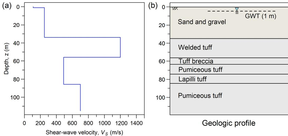
**Figure 2.** Profiles of (a) shear-wave velocity and (b) stratigraphy at KiK-net station FKSH11.
